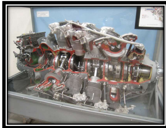
A cutaway of a Pratt & Whitney R-4360 engine.
