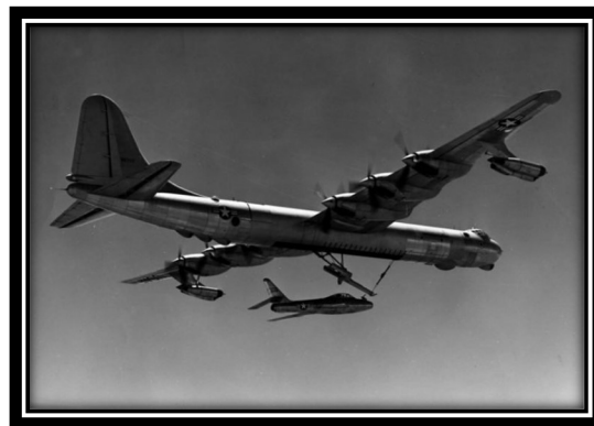
Launching a F-84 from a B-36 in flight
