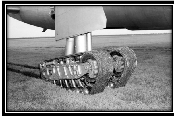
Convair B-36 with experimental tracked landing gear, to reduce ground pressure for soft-field use.
